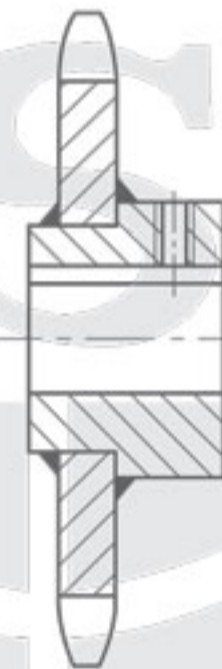
Connection by welding
